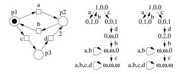
(b) The statement is not true. Indeed, it suffices to use the net from Question 2(b), the example below shows a modified version. It has a deadlock (by firing  $t_1, t_2$ ), but its (unique) coverability graph has two nodes, both with outgoing edges (left figure: net; centre: excerpt of reachability graph; right: coverability graph).
