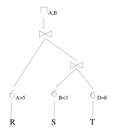
first join S and T, and then join the result with R.
